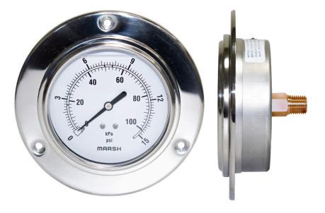
Marsh Instruments Severe Service Liquid Filled Gauges are designed to perform in rugged and harsh environmental conditions, especially where pulsation or vibration is a problem. Liquid Filled Gauges offer a significant cushioning and dampening effect, reducing pointer flutter and lubricating the internals.
