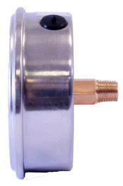
Marsh Instruments Severe Service Liquid Filled Gauges are designed to perform in rugged and harsh environmental conditions, especially where pulsation or vibration is a problem. Liquid Filled Gauges offer a significant cushioning and dampening effect, reducing pointer flutter and lubricating the internals.
