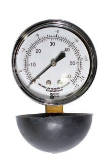
The Marsh Instruments Vacuum Cleaner Test Gauge is designed to test the amount of vacuum generated by a vacuum cleaner to ensure proper operation and to check for leaks or other problems. The Vacuum Cleaner test gauge features a reliable Marsh Instruments Low Pressure Diaphragm Gauge available in several ranges, as well as a rubber plug/fitting designed to fit various different vacuum cleaner hoses and connections.
