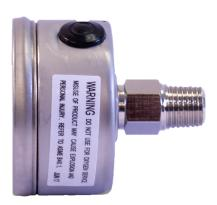
Marsh Instruments Severe Service Liquid Filled Gauges are designed to perform in rugged and harsh environmental conditions, especially where pulsation or vibration is a problem. Liquid Filled Gauges offer a significant cushioning and dampening effect, reducing pointer flutter and lubricating the internals.
