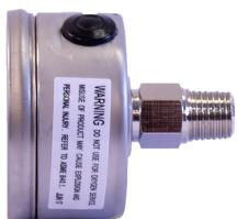
Marsh Instruments Severe Service Liquid Filled Gauges are designed to perform in rugged and harsh environmental conditions, especially where pulsation or vibration is present. Liquid Filled Gauges offer a significant cushioning and dampening effect, reducing pointer flutter and lubricating the internals.
