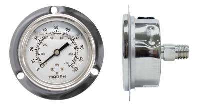
Marsh Instruments Severe Service Liquid Filled Gauges are designed to perform in rugged and harsh environmental conditions, especially where pulsation or vibration is a problem. Liquid Filled Gauges offer a significant cushioning and dampening effect, reducing pointer flutter and lubricating the internals.
