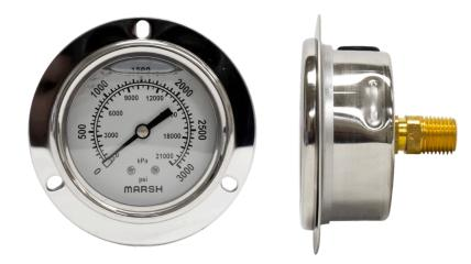
Marsh Instruments Severe Service Liquid Filled Gauges are designed to perform in rugged and harsh environmental conditions, especially where pulsation or vibration is a problem. Liquid Filled Gauges offer a significant cushioning and dampening effect, reducing pointer flutter and lubricating the internals.
