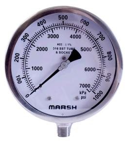
Marsh Instruments Severe Service Liquid Filled Gauges are designed to perform in rugged and harsh environmental conditions, especially where pulsation or vibration is a problem. Liquid Filled Gauges offer a significant cushioning and dampening effect, reducing pointer flutter and lubricating the internals.
