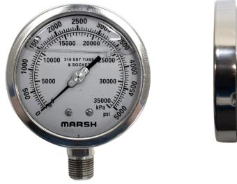
Marsh Instruments Severe Service Liquid Filled Gauges are designed to perform in rugged and harsh environmental conditions, especially where pulsation or vibration is a problem. Liquid Filled Gauges offer a significant cushioning and dampening effect, reducing pointer flutter and lubricating the internals.
