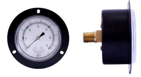
Low Pressure Gauges from Marsh Instruments incorporate a diaphragm element allowing for accurate low-pressure readings in support of a variety of applications, with ASME Grade A 2/1/2% accuracy for ranges above 30" of water. Available ranges include vacuum and pressure in inches of water, ounces per square inch, kilopascals, and millimeters of mercury.
