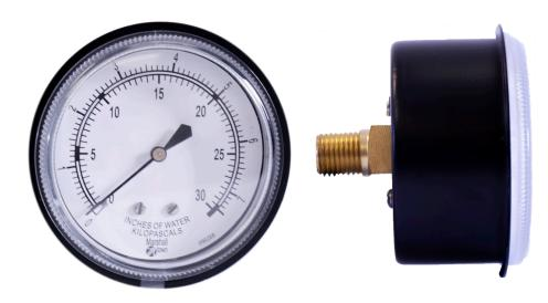
Low Pressure Gauges from Marsh Instruments incorporate a diaphragm element allowing for accurate low-pressure readings in support of a variety of applications, with ASME Grade A 2/1/2% accuracy for ranges above 30" of water. Available ranges include vacuum and pressure in inches of water, ounces per square inch and millimeters of mercury.
