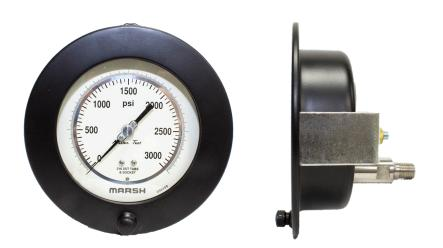
The Marsh Instruments Test Gauge is designed with a black painted steel housing and 316 stainless steel tube and socket to meet the demanding service needs of various test gauge applications. Accuracy is 0.5% of full span. A highly polished integral mirror is positioned between the two graduation arcs on the dial face. The knife-edge pointer is reflective so that, when the pointer and its reflection are in alignment, parallax is virtually eliminated and a true dial reading is assured.
