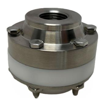
The Model DSP Diaphragm Seal features corrosion resistant PTFE or PVC lower housing with PTFE diaphragm. It is compatible with up to 4" dial pressure gauges from 30 psi up to a maximum operating pressure of 300 psi.
