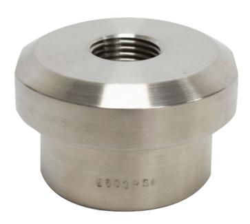
The Model 13040 All Welded Seal is designed for up to to  $4 \frac{1}{2}$ " bourdon tube gauges with pressure ranges from vacuum to 1000 psi. Available in all 316 Stainless Steel or Hastelloy C process housing and diaphragm, with threaded connections. Optional flushing connections also available.
