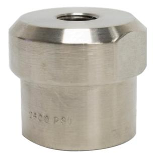
The Model 13000 Mini Welded Seal is designed for up to to  $3 \frac{1}{2}$ " bourdon tube gauges with a minimum range of 0-60 psi. The maximum operating pressure is 2,500 psi at 100°F. Available in all 316 Stainless Steel or Hastelloy C process housing and diaphragm.
